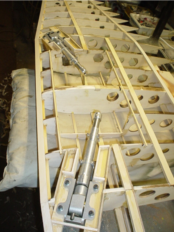
Retracts are temporarily fitted to ensure correct alignment.
