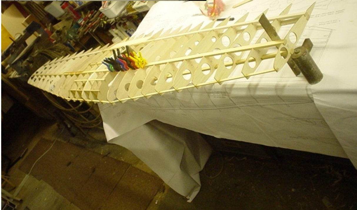
Joining the pieces. The centre section is held down on the bench with weights and then the wing tips are raised for the required amount of dihedral. Plywood dihedral braces are inserted, top and bottom, alongside main and auxiliary spars and epoxied and clamped in place.
